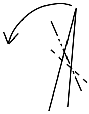
19. First crimp down to form the head.
